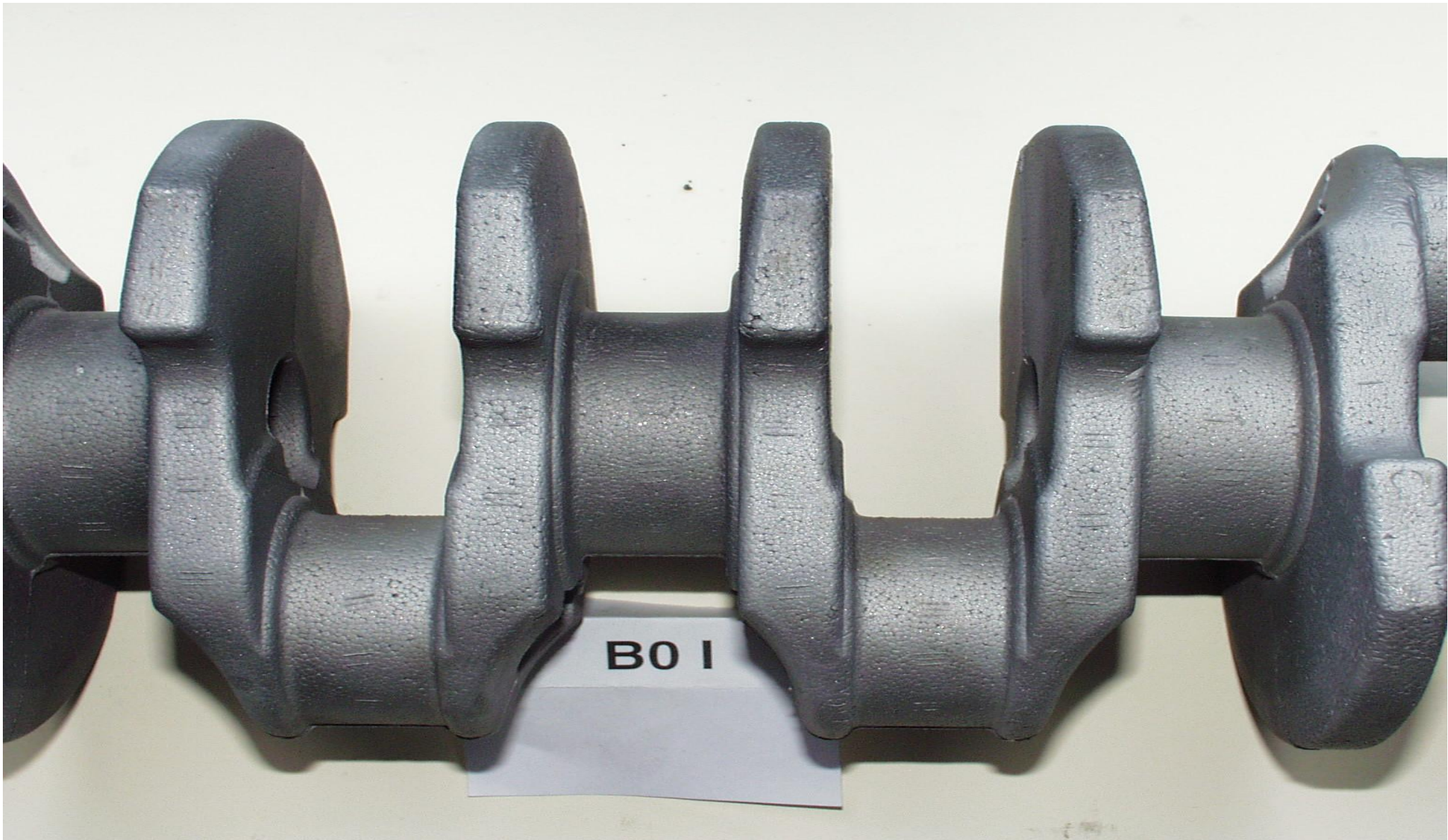
GJS- crank shaft as cast
